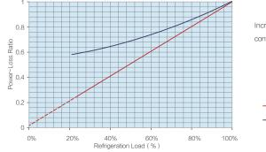
Increased efficiency in part load by frequency control compared to mechanical slider operation
